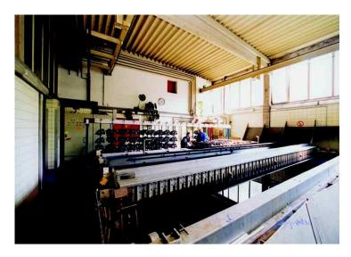
Figure 5: The anodizing plant
