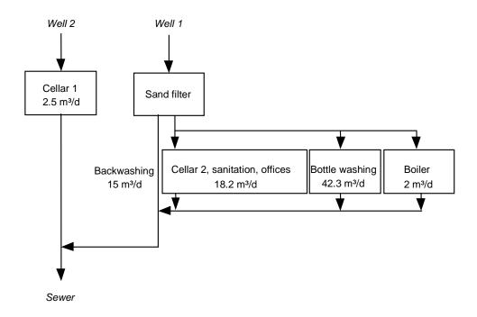
Figure 1: Flow sheet of water in Znovin
